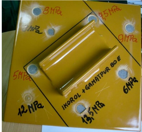
Figure 7. Panel No. 3 (BSa2.5 condition) – pull off results, no cuts around the punches (black) – with ikorol ® : 6 and 13.5 MPa, without ikorol ® : 8 and 12 MPa; with cuts around the punches (red) – with ikorol ® : 5 and 7.5 MPa, without ikorol ® : 8 and 9 MPa
