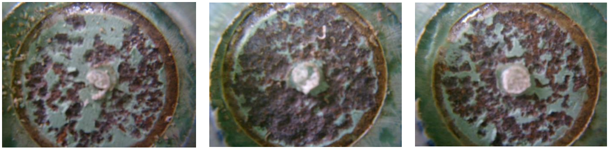
Figure 10. Panel No. 7 (untreated sample, C condition) – the appearance of areas after stamps being torn off, cohesive detachment on the surface of approx. 90%
