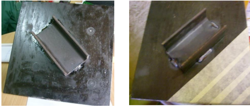
Figure 2. Panels No. 1 (left) and no. 2 (right) (condition B) – painted with ikorol shield
