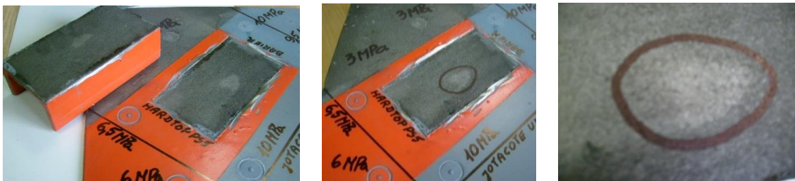
Figure 14. Panel No. 6 (BSa2.5 condition) – appearance after the seasoning and cutting the channel section (C-profile) on welds. Under the C-profile and on the C-profile from the bottom the penetration of ikorol ® on approx. 95% of the surface is visible. The non-penetrated fragment is marked
