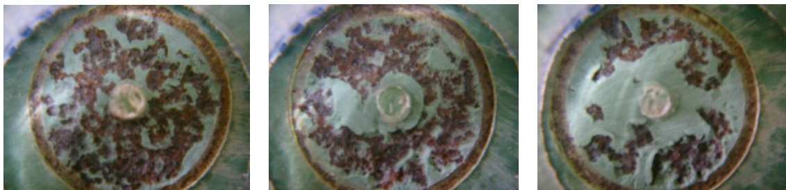
Figure 11. Panel No. 8 (sample cleaned manually with a wire brush, CSt1 condition) – the appearance of areas after stamps being torn off, cohesive detachment on the surface of approx. 60–70%
