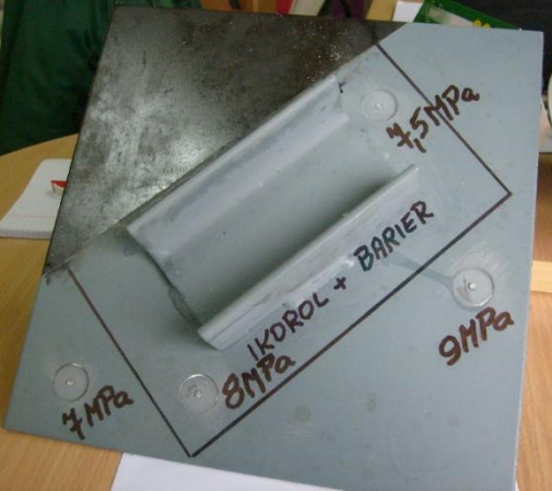
Figure 4. Panel No. 2 (condition B) – pull off results, with ikorol ® : 7.5 and 8.0 MPa, without ikorol ® : 7 and 9 MPa
