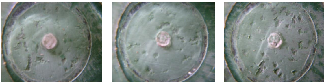
Figure 12. Panel No. 9 (sample blasted with a copper slag, CSt2.5 condition) – the appearance of areas after stamps being torn off, cohesive detachment on the surface of approx. 5%
