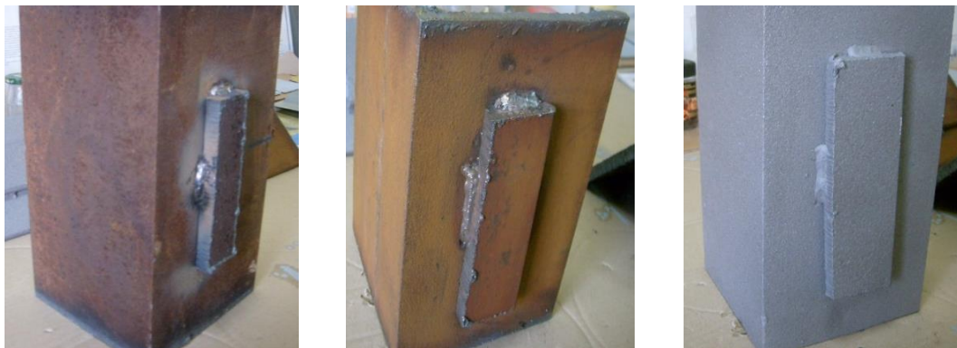
Figure 3. Appearance of heavily corroded samples – No. 7 (left) (condition C) without any cleaning, No. 8 (middle) (condition CSt1) after manual cleaning with a wire brush, No. 9 (right) (condition CSt2.5) after blasting with copper slag
