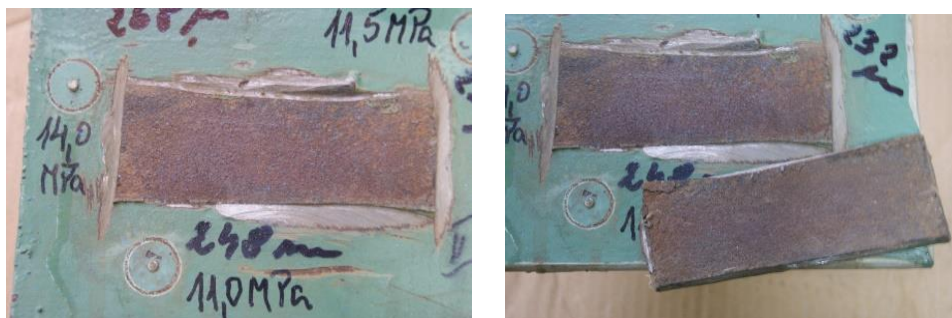
Figure 16. Panel No. 8 (CS1 condition) (left), Panel No. 9 (CSa2.5 condition) (right) – appearance of the surface after the seasoning and cutting off a flat bar
